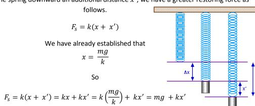
In our free body diagram at this point, we have spring force upward and gravitational force downward, so the net force is
